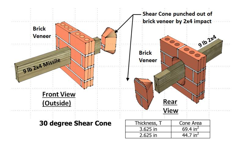
The 2.625" brick has 64% of the shear cone area of the 3.625" brick as tested. So we can expect it to absorb 64% of the impact energy or 1531 Joules. That gives a velocity for the 9 lbm 2x4 of 60.8 mph.
