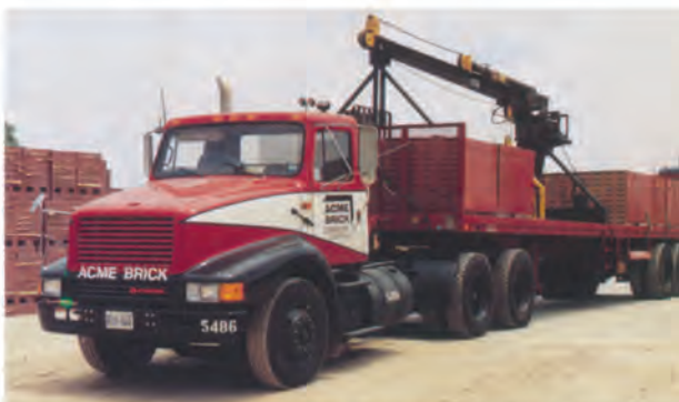
Top: Acme delivery truck parked outside the company headquarters building in 1963. Note the tandem trailer, brick packaging system, and crane to off load the brick.
