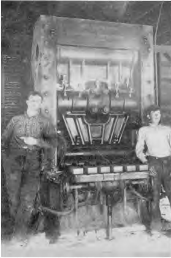
Above: Acme Pressed Brick Company's new six mold Boyd press when it was installed in 1894.
