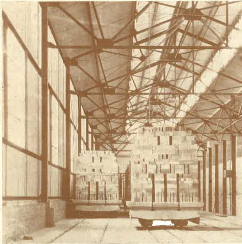
NEW TUNNEL KILN EQUIPMENT, ACME BRICK COMPANY'S PERLA PLANT Predetermined Colors—Large Volume Production
