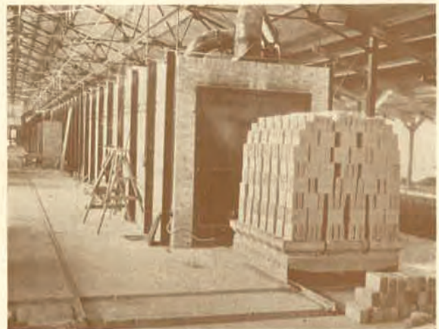
The Tunnel Kiln, and a Kiln Car Loaded with Acme Brick
