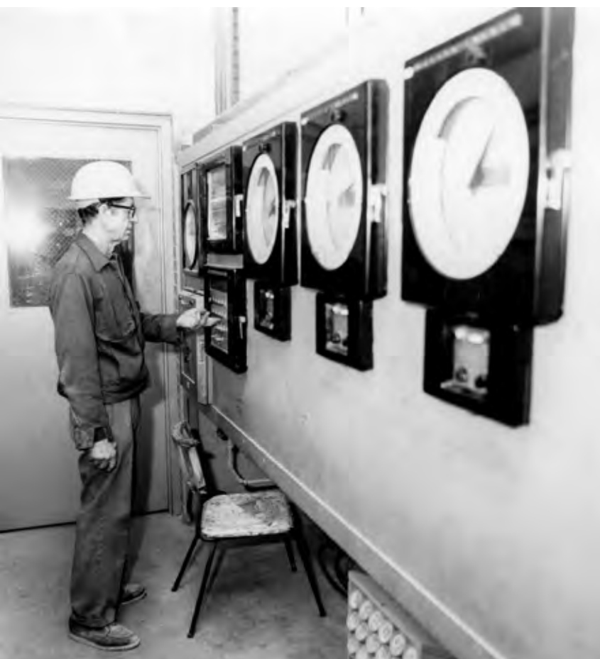
A burner at an Acme Brick Plant checks kiln temperature control, circa the 1960s.
