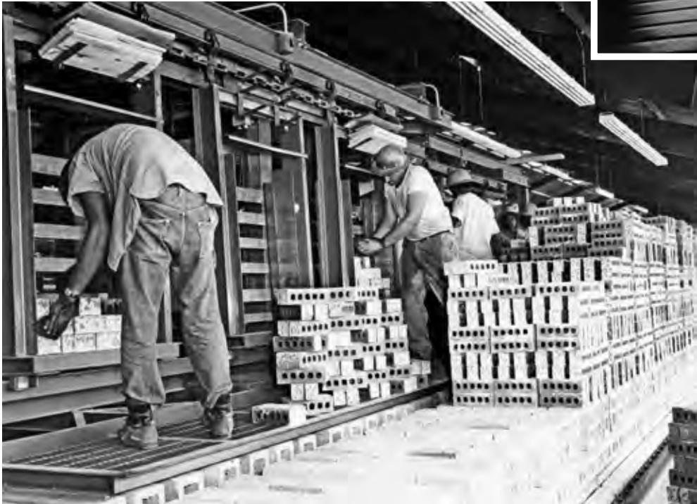
Dehacking brick in the 1970s; the implementation of Occupational Safety and Health Administration (OSHA) regulations during the decade required workers to don hard hats and safety glasses when on the line.
