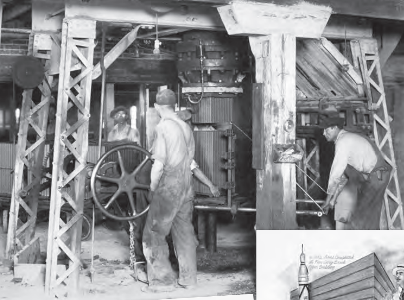
Workers extruding clay structural tile at the Denver Plant in the 1930s.
