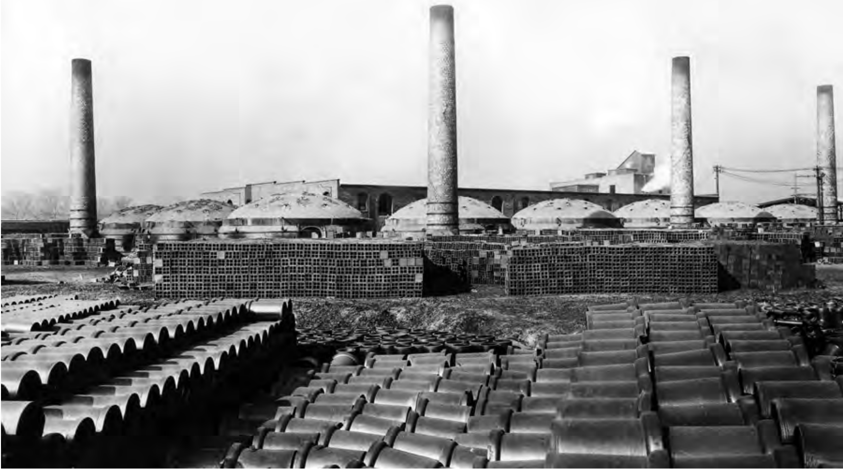
Much of the output at the company's Denver Plant in the 1920s was sewer pipe (foreground) and drain tiles (background).
