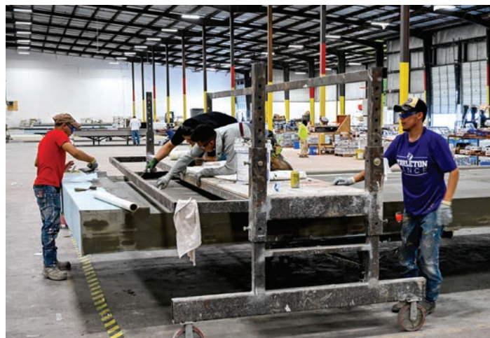
BakerTriangle employees prepare a prefab wall panel for Fred Hill Elementary School. Thinset mortar is applied to the panel in preparation for the laying of thin brick slips.
