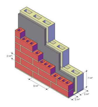
King Size Brick and 4" Light Weight Block, Cavity Wall
