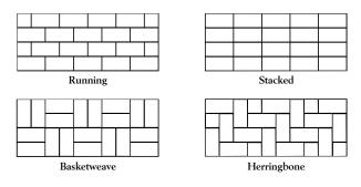
NOTE: For basketweave pattern, a full  $4" \times 8"$  unit must be used unless the joints are grouted.
