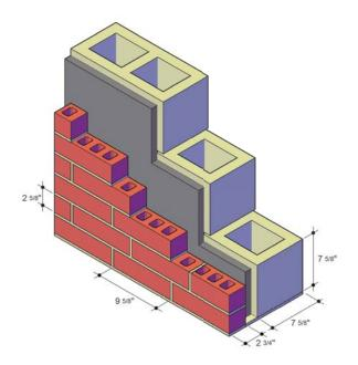
King Size Brick and 8" Light Weight Block, Cavity Wall
