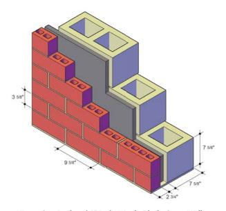
Estate Size Brick and 8" Light Weight Block, Cavity Wall
