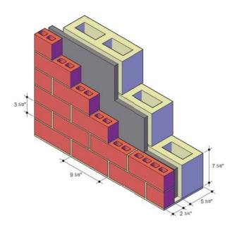
Estate Size Brick and 6" Light Weight Block, Cavity Wall
