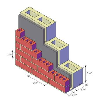
King Size Brick and 6" Light Weight Block, Cavity Wall
