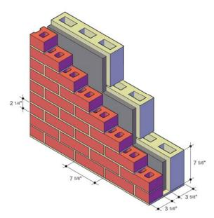
Modular Face Brick and 4" Light Weight Block, Cavity Wall
