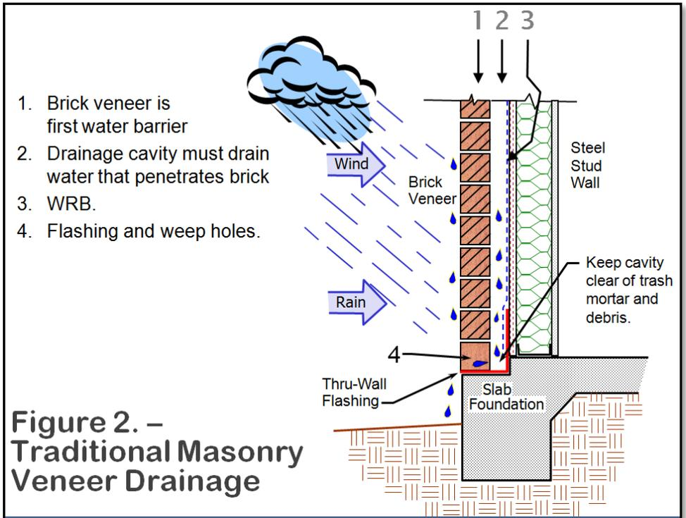
**Figure 2. – Traditional Masonry Veneer Drainage**
