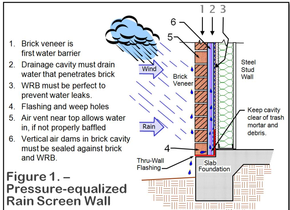
**Figure 1. – Pressure-equalized Rain Screen Wall**
