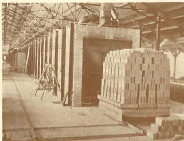
The Tunnel Kiln, and a Kiln Car Loaded with Acme Brick
