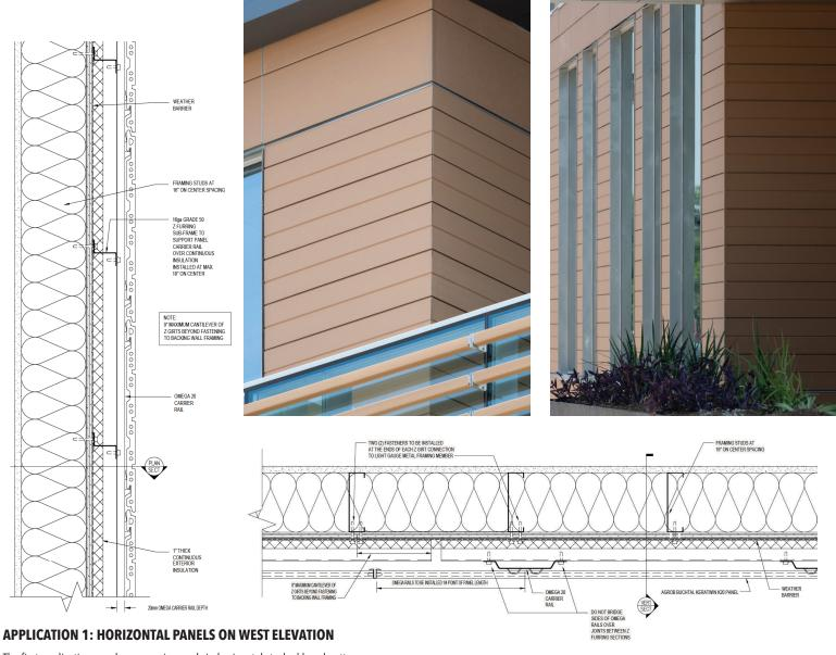
The first application employs ceramic panels in horizontal stacked bond patterns. Large smooth-faced expanses and smaller grooved panels create a sophisticated wainscot effect.
