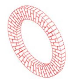
For Circular Arches, the arch pieces need to be tapered to maintain a consistent width mortar joint. If the pieces are not tapered, then the mortar joint will need to be tapered, which is less desirable. As the masonry opening gets larger, a field brick may be the best option, because the taper of the arch piece is less discernible. Send us your arch details and let us determine what is needed for the best application in these situations.
