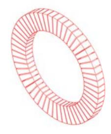
For Circular Arches, the arch pieces need to be tapered to maintain a consistent width mortar joint. If the pieces are not tapered, then the mortar joint will need to be tapered, which is less desirable. As the masonry opening gets larger, a field brick may be the best option, because the taper of the arch piece is less discernible. Send us your arch details and let us determine what is needed for the best application in these situations.
