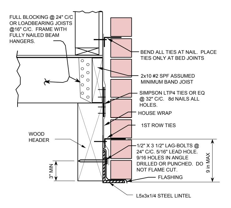
Fig 2. - WOOD HEADER AND STEEL ANGLE LINTEL
