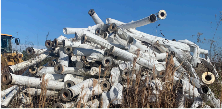
Pile of discarded filters with steel cages
