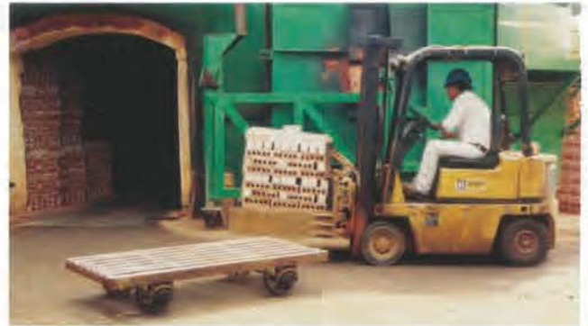
Filling a thin clad kiln at Bridgeport with dried brick prepared for burning.
