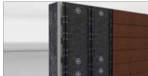
Mount the T-profile with approved fastening means
