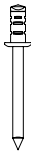
Article 658 Al blind rivet, bright Weight: 1.3 kg / box Nominal dimensions: 4.8 x 10 mm Box contents: 500 pieces for the fastening of Omega profile and OmegaS
